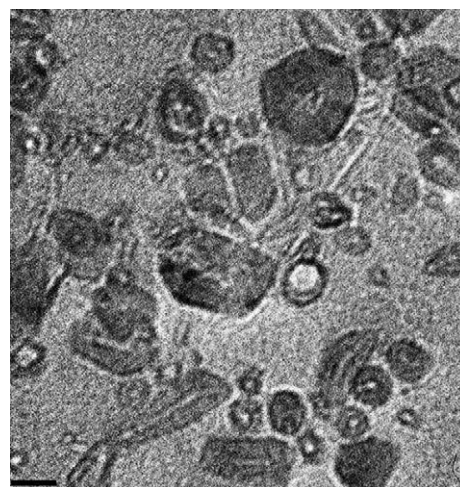
Figure 4. Purified (annealing, HNO 3 /microwave, SCW, annealing) CNOs (30 Å). Scale bar represents 20 nm.
